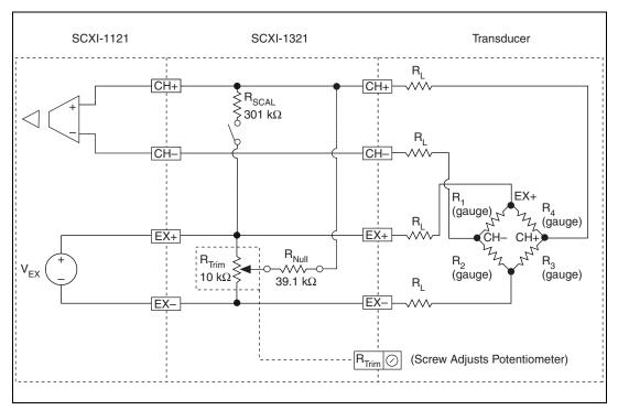
Figure 5. Full-Bridge Nulling Circuit
